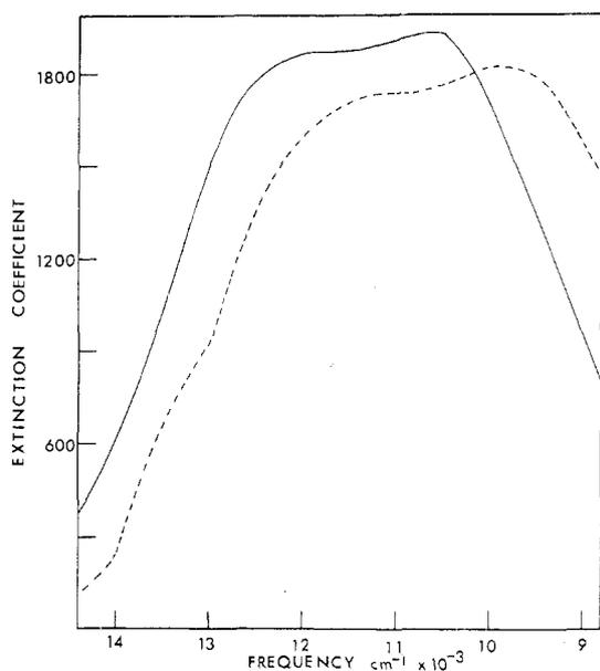
Figure 3.—Absorption spectrum of  $\text{Cu}_4\text{OCl}_6(\text{TPPO})_4$  in acetone (solid line) and as the solid in a potassium bromide pellet (broken line). The extinction coefficients refer to the solution spectrum; the solid spectrum is on an arbitrary scale.
